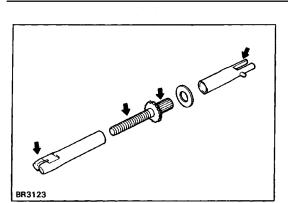
(b) Apply high temperature grease to the adjuster bolt threads and ends.
