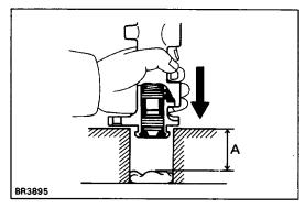
(c) Place a rag and two wooden blocks on the work table, and lightly tap the cylinder flange against the block edges until the No.2 piston drops out of cylinder.
