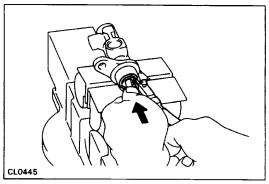
3. INSTALL PUSH ROD ASSEMBLY WITH SNAP RING
